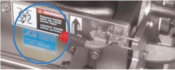
Typical Nameplate showing Serial Number location. Serial no. should be provided when consulting the factory
